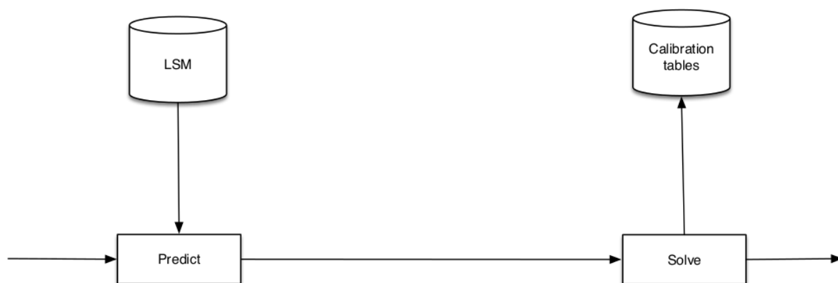
Figure 2: The Real Time Calibration pipeline RCAL. Visibility data are input at DFT and Snapshots. The output data are the calibration solution send to the Calibration Tables.
